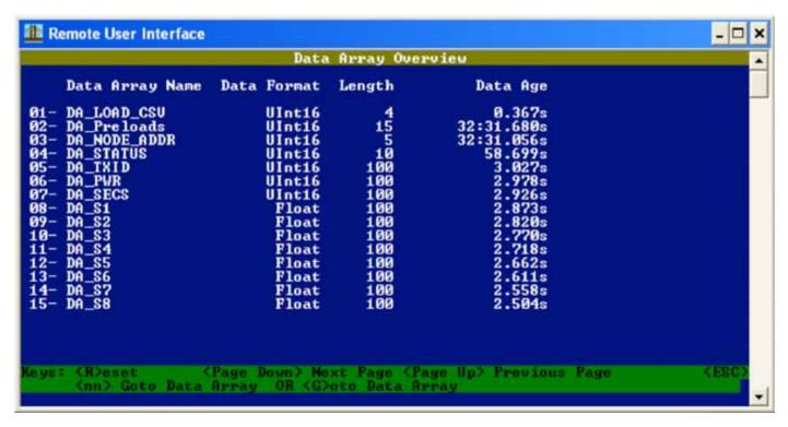
This screen shows all the data arrays available on the FieldServer. The WSG writes data into the following arrays:
