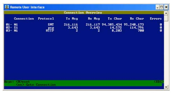
This screen is useful for verifying error-free connectivity across the desired protocol. In the screen above, the FieldServer is being used as an XML/HTTP server for the internal data arrays.
