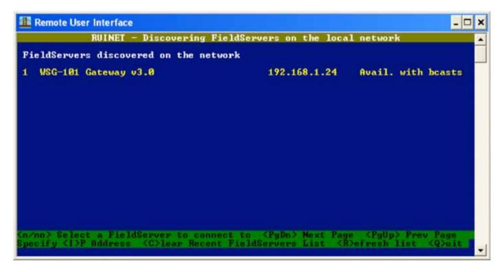
Initially, a FieldServer device's IP address is 192.168.1.24. If the host network does not match this default setting, an RS-485 or FTT-10 model will be allow communication through RUInet using broadcasts, as seen in Figure 2.
