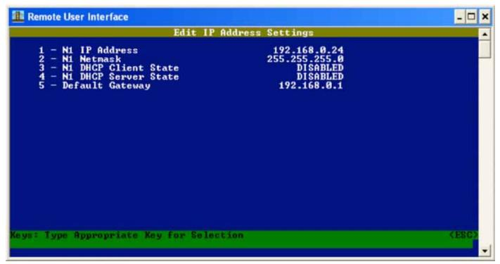
This option is used to change the IP address of the FieldServer. The FieldServer in the screen above has had it's IP address changed to match the host network.
