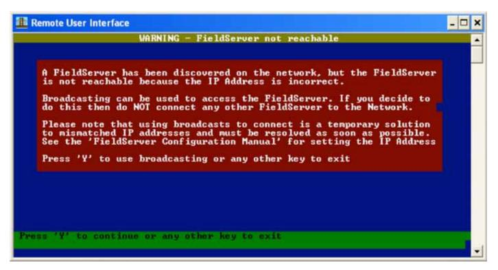
This is not preferable, but allows the user to change the IP of FieldServer device to match the host network.
